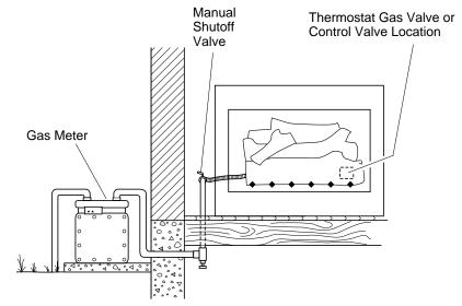
Figure 14 - Checking Gas Joints
